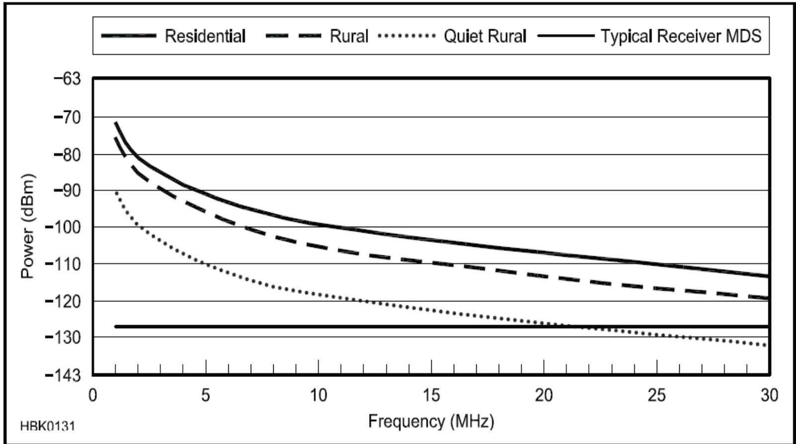
Fig 1 — Typical noise levels versus frequency for various environments. (Man-made noise in a 500-Hz bandwidth, from Rec. ITU-R P.372.7, *Radio Noise*)
