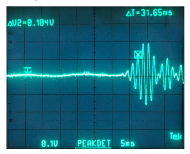
Latency varies with the type of architecture, and it generally increases with narrower filter bandwidths. Analog transceivers generally have latency under 10ms, while the better DSP variants have latency under 20ms. Some transceivers have latency between 50 and 170ms depending on design trade-offs between filter shape factor and the signal delay. For best QSK performance a latency of 20m or less is desirable.
