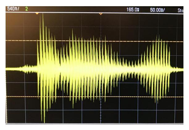
CW overshoot at 30 watts key down. 30 watts was at the right edge of the "dit".
