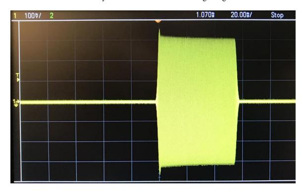
The key line timing is acceptable for a QSK capable linear amplifier. Unless there is a menu setting to adjust for slower T/R relays in non-QSK amps, hot switching may occur on CW and SSB on the initial power output. The "key-up" delay is adequate. Key down delay is about 14ms, and key up is about 3ms.
