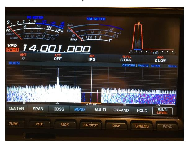
There is no dedicated power output knob, which is inconvenient when adjusting drive to a linear amplifier. This requires a button push, a push on the multi-function knob, then selecting the power output function on a very busy menu, and finally adjusting output power with the multi-function knob. This can be assigned to the C. S. button, but takes 3 functions: Push C.S. button, adjust with sub-RX VFO dial, push C.S. button again.
