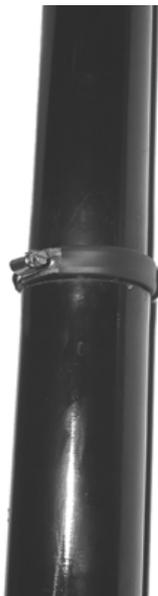
The **first** clamp (50-70mm diameter) is mounted at the **bottom end of the second tube segment**. Here it will act as a stopper and prevent the second tube from sliding downwards into the first tube segment. The rubber padding safely protects the mast against any damage from the clamps.
