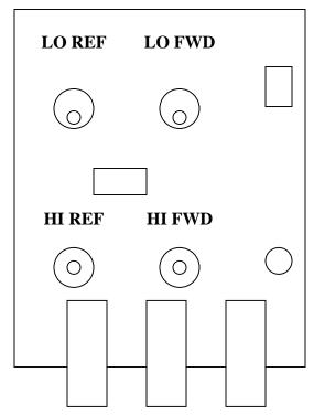
Figure 2: PCB Layout and Trim Pot Location
