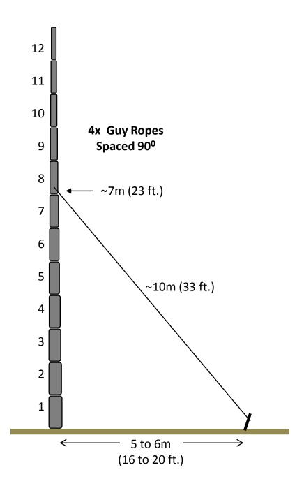
Attach 3 (preferably 4) guy lines to the pole above segment number 7 (height = 7m). We recommend a guying distance from the pole of 5 to 6m. This results in a guy line Length of approx. 10m. You will need 4x10m = 40m of 2mm Kevlar here rope. We recommend purchasing one roll (50m) of Kevlar rope and cutting it into 4 pieces, each 12m long. NOTE: 1m = 3.3 ft.
