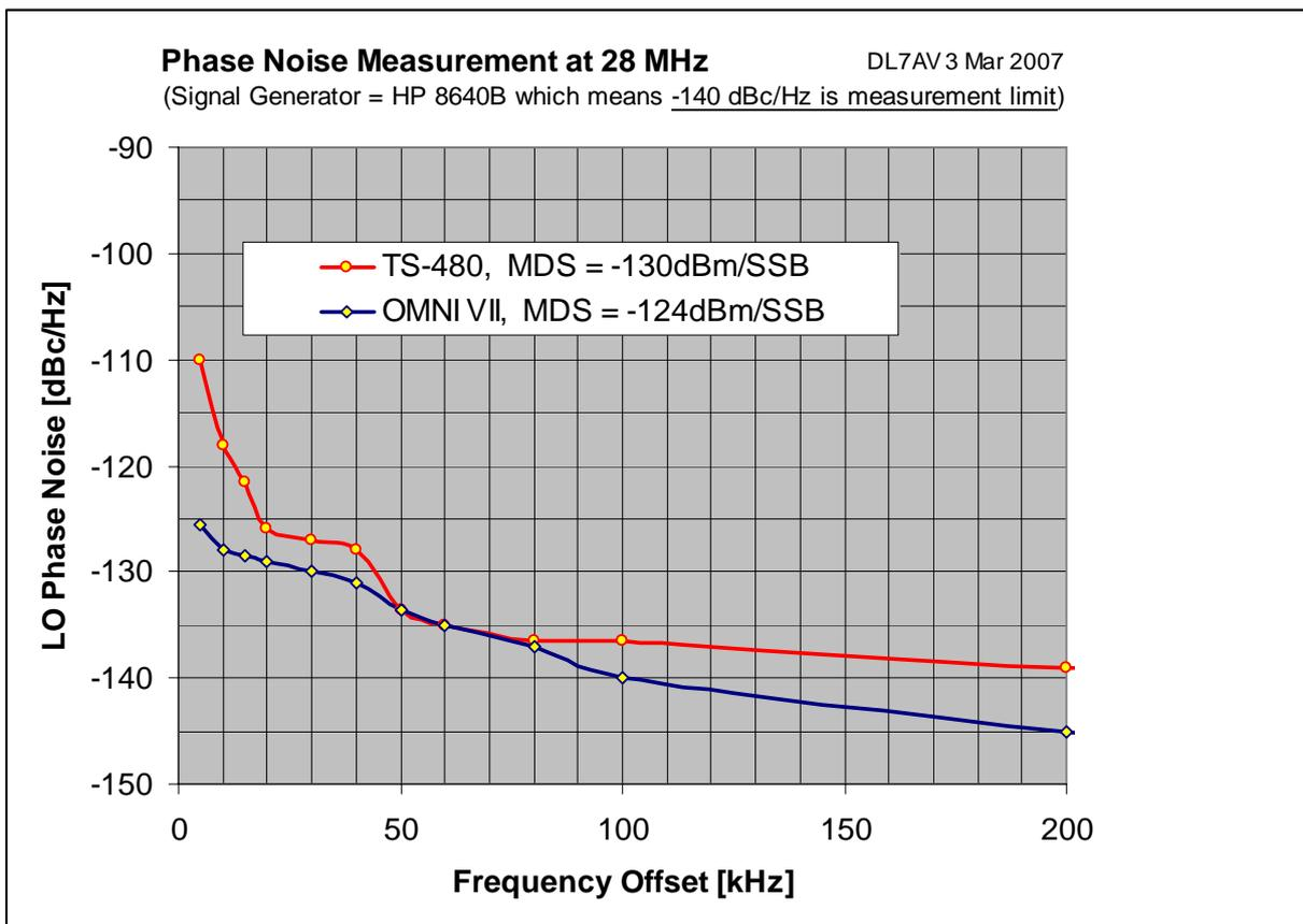
Note: "MDS" = minimum discernable signal (values shown are just for info, & not associated with this graph. The OMNI VII was measured with preamp OFF)
