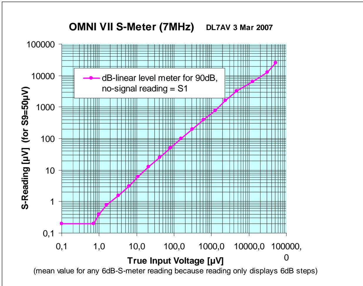
As can be seen, the S-meter is accurate enough to be used for field strength measurements, if you can accept that the increments are in full S-units. This is possibly the only rig currently on the market that can read accurately all the way down to S-2.
