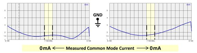
Again with zero measurable CMC, the single-core balun has a distorted SWR curve. I am still searching for an explanation for this! With C3, regardless of whether it is grounded or not, the SWR curves of the dual-core balun look great; just like the coax coming straight down the pole.
