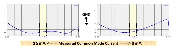
With almost zero CMC, the single-core balun still has a distorted SWR curve. I am still searching for an explanation for this! With C4, regardless of whether it is grounded or not, the SWR curves of the dual-core balun look great; just like when the coax is running straight down the pole.
