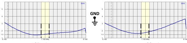
105 mA ← Measured Common Mode Current → 39 mA
