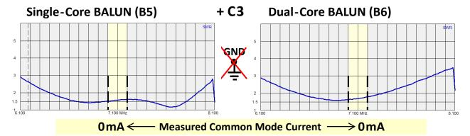
The CMC is gone in both, but the SWR curve on the left is still distorted! (The right is OK.)
