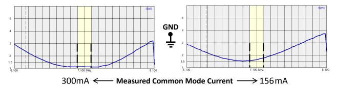
When "grounded", the picture changes on both sides. The curve on the left is what we all dream of at night. But then we wake up. The curve on the right has returned to its original shape, but is still showing a lower SWR than the antenna really has. That was one small step in the right direction
