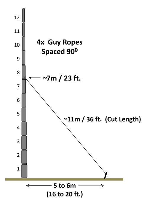
Attach 4 guy lines to the pole above segment number 7 (height = 7m). We recommend a guying distance from the pole of 5 to 6m. This results in a guy line Length of approx. 11m. You will need 4x 11m = 44m of 2mm Kevlar rope. We recommend purchasing one roll (50m) of Kevlar rope and cutting it into 4 pieces, each 12m long. NOTE: 1m = 3.3 ft.
