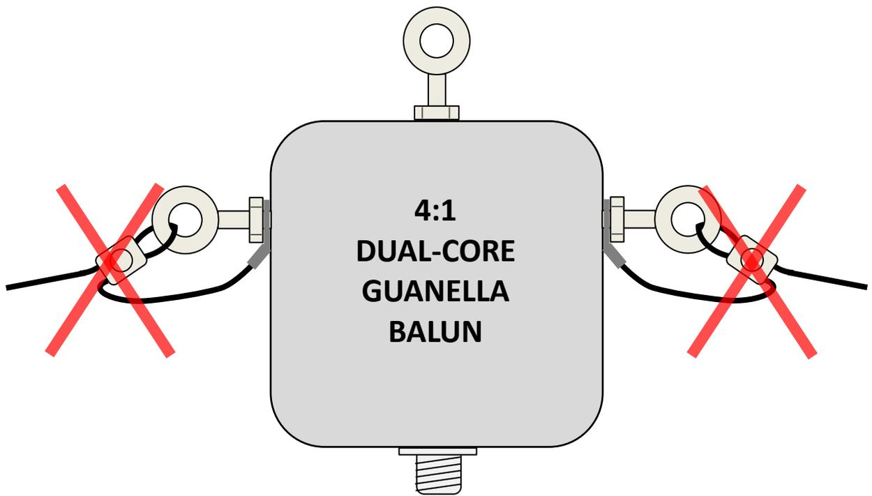
Precise definition of the feedpoint is important for achieving efficient multi-band performance. The traditional method shown above is too ambiguous for this application and difficult to exactly replicate. **DO NOT USE THIS METHOD.**
