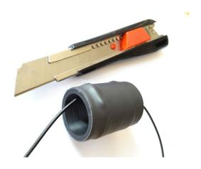
7. Slide a 30 mm piece of 3/1 mm and 30 mm piece of 6/2 mm heat-shrink tubing over the end of the 355 cm CQ-532. Solder a 90° solder lug to the end of the wire. Then slide the 3 mm heat-shrink tubing **against** the solder lug, heat and shrink. Next, slide the 6 mm heat-shrink tubing **over** the solder lug, heat and shrink.
