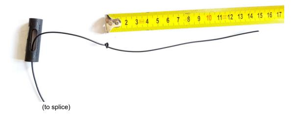
4. Fold back 10cm of wire at the point 5cm away from the knot and fasten with two small wire-ties.
