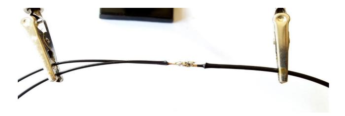
2. Slide a 50mm long piece of 3/1 mm heat-shrink tubing over the splice and heat to shrink. Then slide a 30mm long piece of 6/2mm heat-shrink tubing over the 3/1 mm tubing, heat to shrink. Do this for both ends of the dipole.
