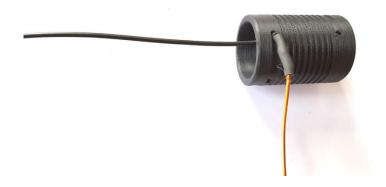
4. Now while pulling the wire tight, wind the copper wire into a coil, such that it fits snuggly into the grooves. When reaching the end of the copper wire, insert the far end of the CQ-532 wire through the hole in the coil form and pull the wire tight, such that the heat-shrink tubing is sitting in the thick groove at the end of the form and the wire does not move on the coil form.
