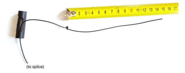
4. Fold back 10cm of wire at the point 5cm away from the knot and fasten with two small wire-ties.
