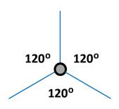
**3** guy ropes at each level, equally spaced by 120 degrees.
