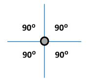
**4 guy ropes** at each level, equally spaced by 90 degrees.
