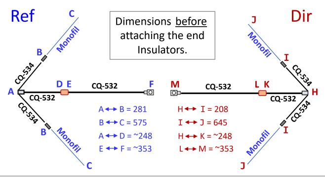
Note: The lengths of the **CQ-532** Wire Radiator segments may vary by a cm, depending on the size of the splices. This can be compensated for in the loops at the ends of the top-hat wires.
