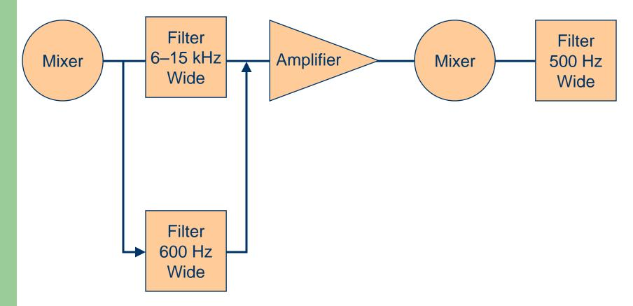
This keeps the undesired strong signals from progressing down stream to the next stages
