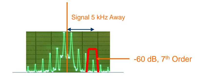
IF Filter vs. Adjacent Signal and IMD Splatter
