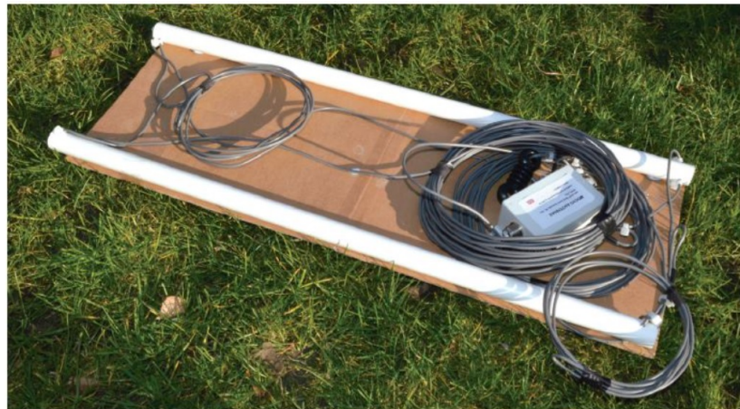
The starting point of the antenna is the classic off centre fed dipole.
