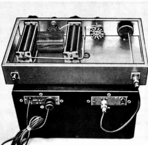
Fig. 13-16—An example of how the antenna coupler can be built. In this case the components are installed in a 10 × 17 × 3-inch aluminum chassis that serves as the support for the transmitter. An r.f. ammeter (right) is used as an output indicator. (W4UWA/DL4, QST, November, 1958).
